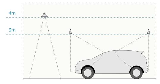
Installation principle without suspended ceiling
