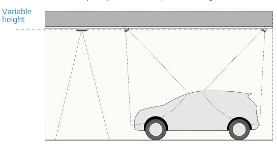
Installation principle with suspended ceiling
