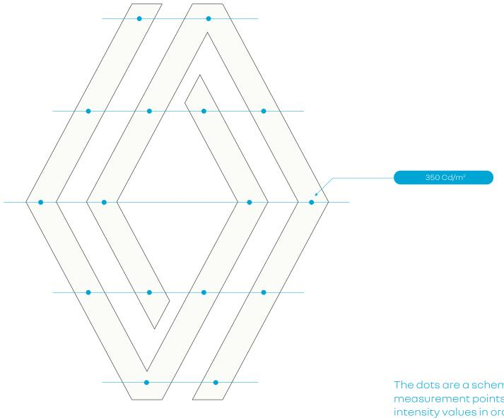
The dots are a schematic representation of the measurement points that should present similar light intensity values in order to obtain even lighting across each of the letters of the Renault word.
