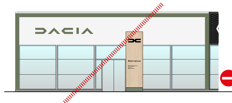
The entrance totem is not adapted to the height of the facade
