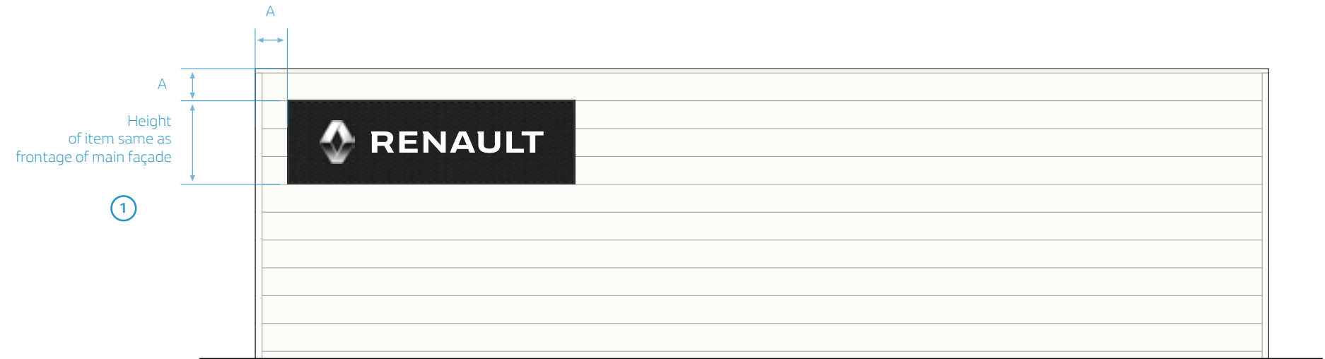
Positioning on left side of blind façade
